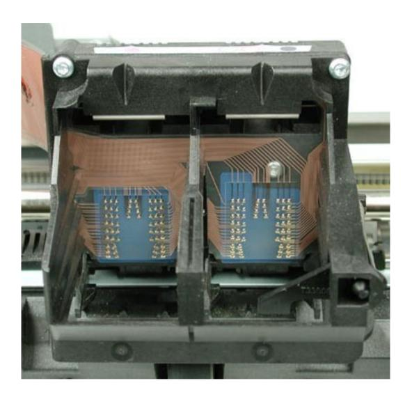
The print head stepper motor moves the print head assembly (print head and ink cartridges) back and forth across the paper.
